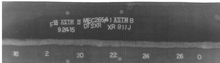
.75" Thick BFW valve weld, 4-90 second exposures (6-9 minute exposures with conventional RT)
